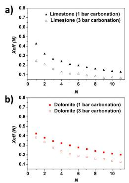
Figure 8. Multicycle effective conversion data for (a) natural limestone and (b) dolomite, as a function of the number of carbonation/calcination cycles, under atmospheric and high-pressure carbonation [79].
