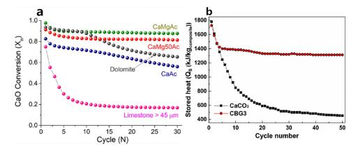
Figure 10. (a) Multicycle CaO conversion of different sorbents under energy storage conditions and (b) the long-term cyclic stored heat performance of pure CaCO<sub>3</sub> and CaCO<sub>3</sub>/graphite [93].
