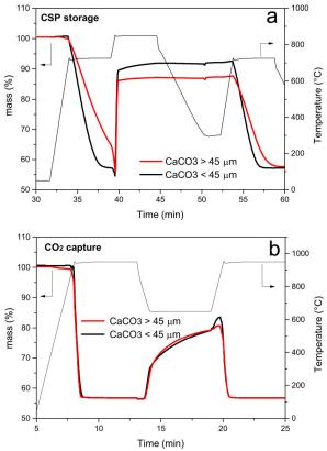
Figure 5. Time evolution of temperature and sample weight for the first carbonation cycle of CaCO<sub>3</sub> using different particle sizes, under (a) CaL-CSP and (b) CaL-CO<sub>2</sub> capture conditions [71].
