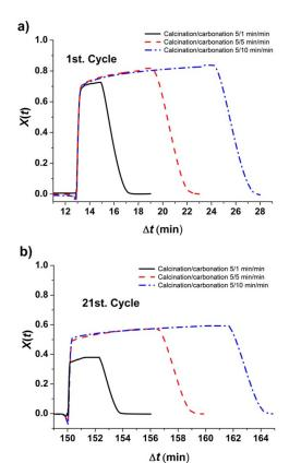
Figure 6. Time evolution of CaO conversion during the (a) first and (b) 21<sup>st</sup> cycle for carbonation/calcination tests carried out under CaL–CSP conditions [72].
