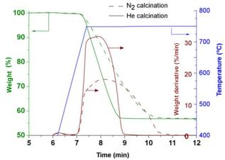
Figure 7. The time evolution of weight, weight derivative, and temperature during the decomposition of limestone under either a pure  $N_2$  or He atmosphere [72].
