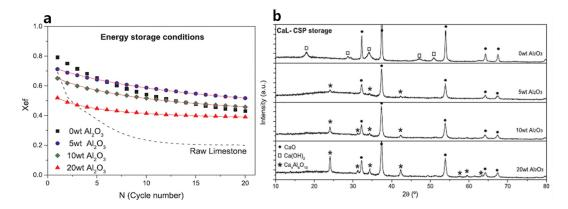
Figure 9. (a) Multicycle activity of milled limestone and Al<sub>2</sub>O<sub>3</sub>/CaCO<sub>3</sub> mixtures with different Al<sub>2</sub>O<sub>3</sub> amounts and (b) X-ray diffractograms of milled limestone and composites after the 20<sup>th</sup> CaL cycle under energy storage conditions [90].
