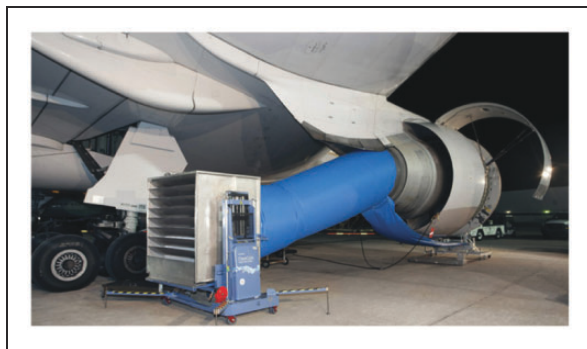
Figure 4. On-wing compressor washing with capture of effluents. 8
