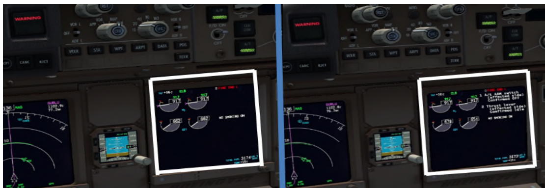
Figure 3. The traditional EICAS (left); and the “integrated” EICAS design (right)
