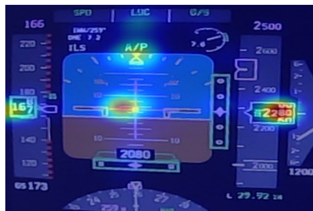
Figure 1. Pilot’s visual scan patterns shown as heatmap reflected to attention distributions among Primary Flight Display (PFD)
