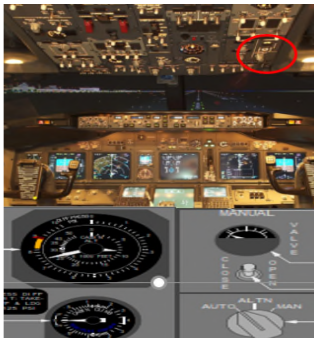
Figure 3. The position of B-737 cabin pressurization on the top of right-hand seat in the flight deck shown as red circle
