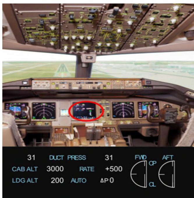
Figure 4. The position of B-777 cabin pressurization in the center of flight deck shown as red circle
