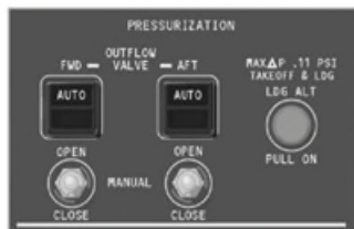
Boeing 777 Cabin Pressurization Control Panel
