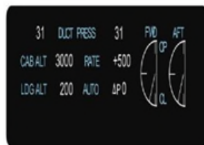
Boeing 777 Cabin Pressurization System Display
