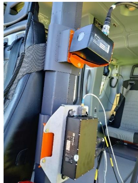
Figure 5: RT-TipTrak (top) and HT-VMU (bottom) mounted to the central pillar on the H135.
