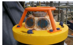
Figure 2: ADCP before installation under water [7]
