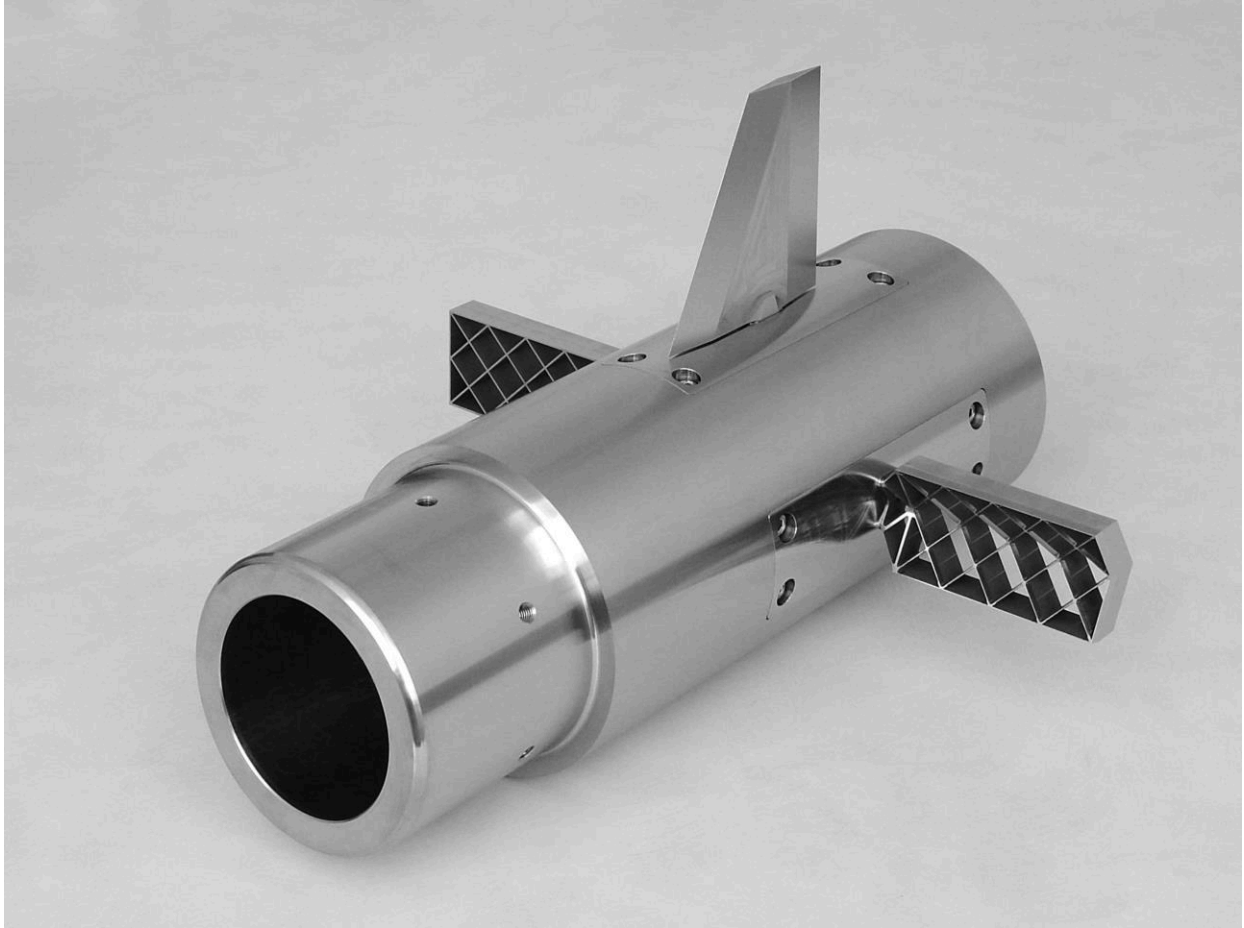
Fig. 2 Picture of the rear part of the ogive-cylinder body with concurrent installation of the baseline grid fin, the planar fin, and the swept-forward grid fin (clockwise from left to right). In the wind-tunnel the holes of the screws were covered by plugs to maintain an aerodynamically smooth surface.
