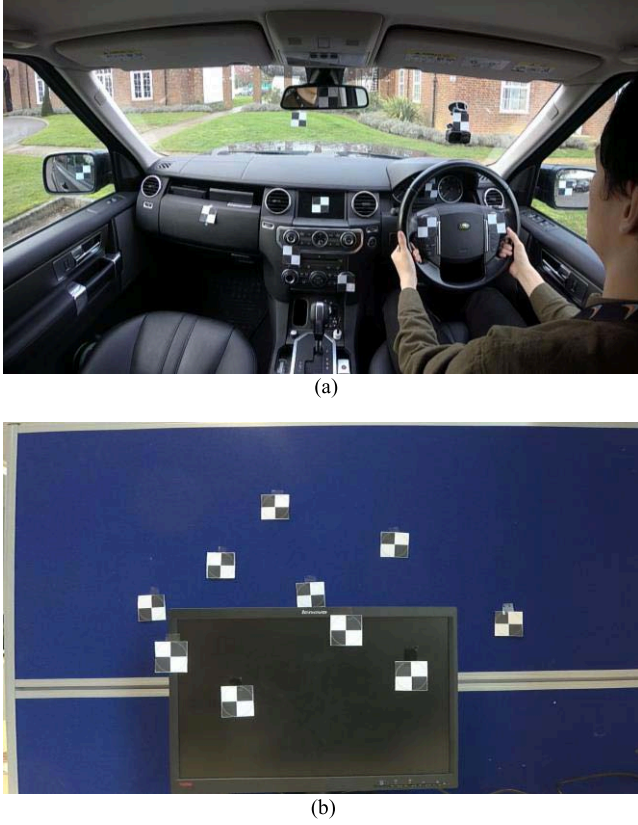
Fig. 2. (a) The spatial distribution of the markers in land rover discovery 4 for the in-vehicle experiment. (b) The spatial distribution of the markers in laboratory for the indoor experiment.
