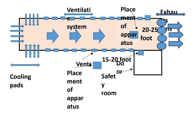
Fig. 1: A representative illustration of the design of an environmentally controlled poultry shed
