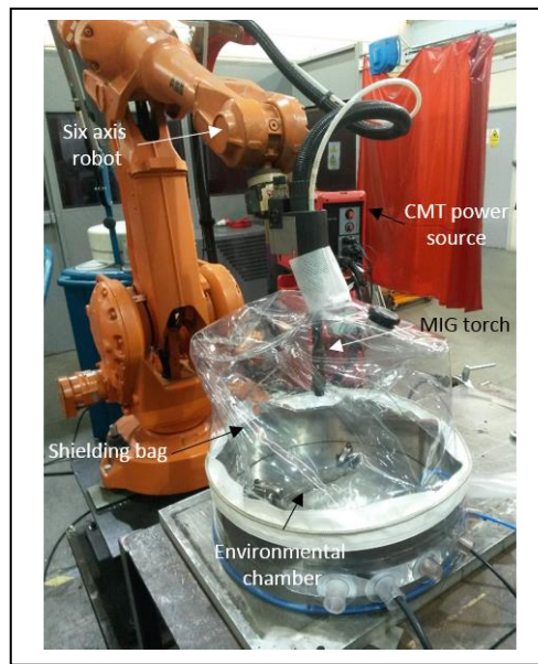
Fig. 2. Experimental set up for the shielding gas assessment.
