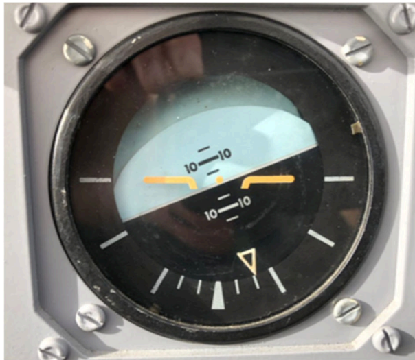
Figure 1. An example of a moving-horizon type AI, as used in this study, displaying a bank to the right.
