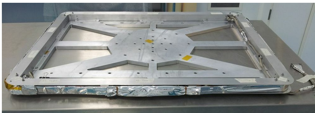
Figure 3.2: Icarus-1 in stowed configuration. The payload is mounted to an aluminium mechanical ground support equipment plate for assembly and test.
