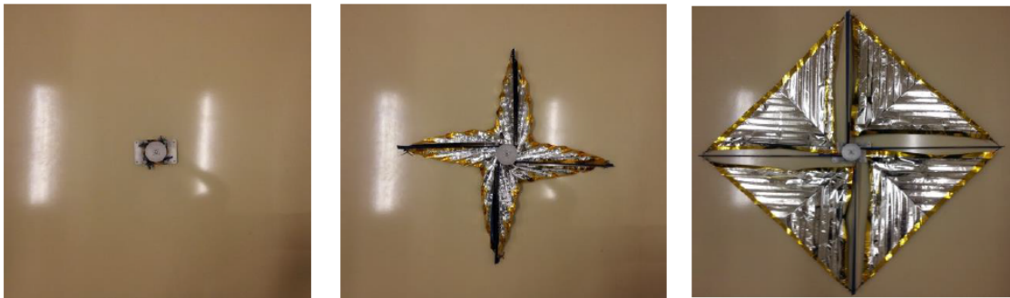
Figure 3.16: Sail deployment process for DOM prototype.
