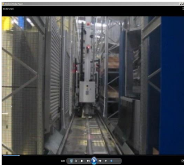
Figure 34 Snapshot of stacker crane video
