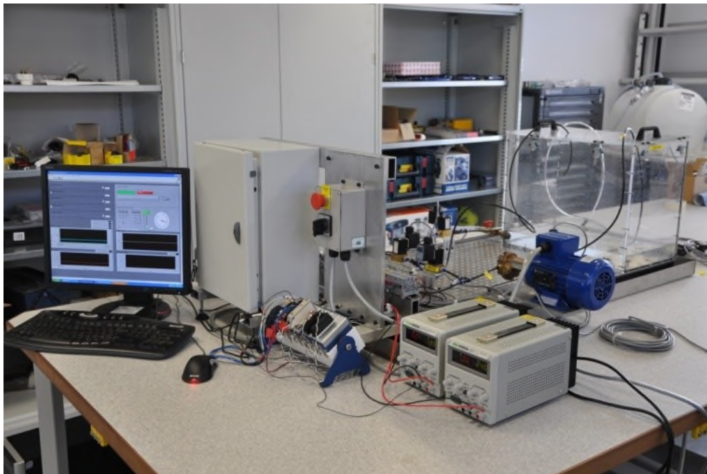
Figure 3-3 Photograph of the fuel rig in the IVHM Centre at Cranfield University
