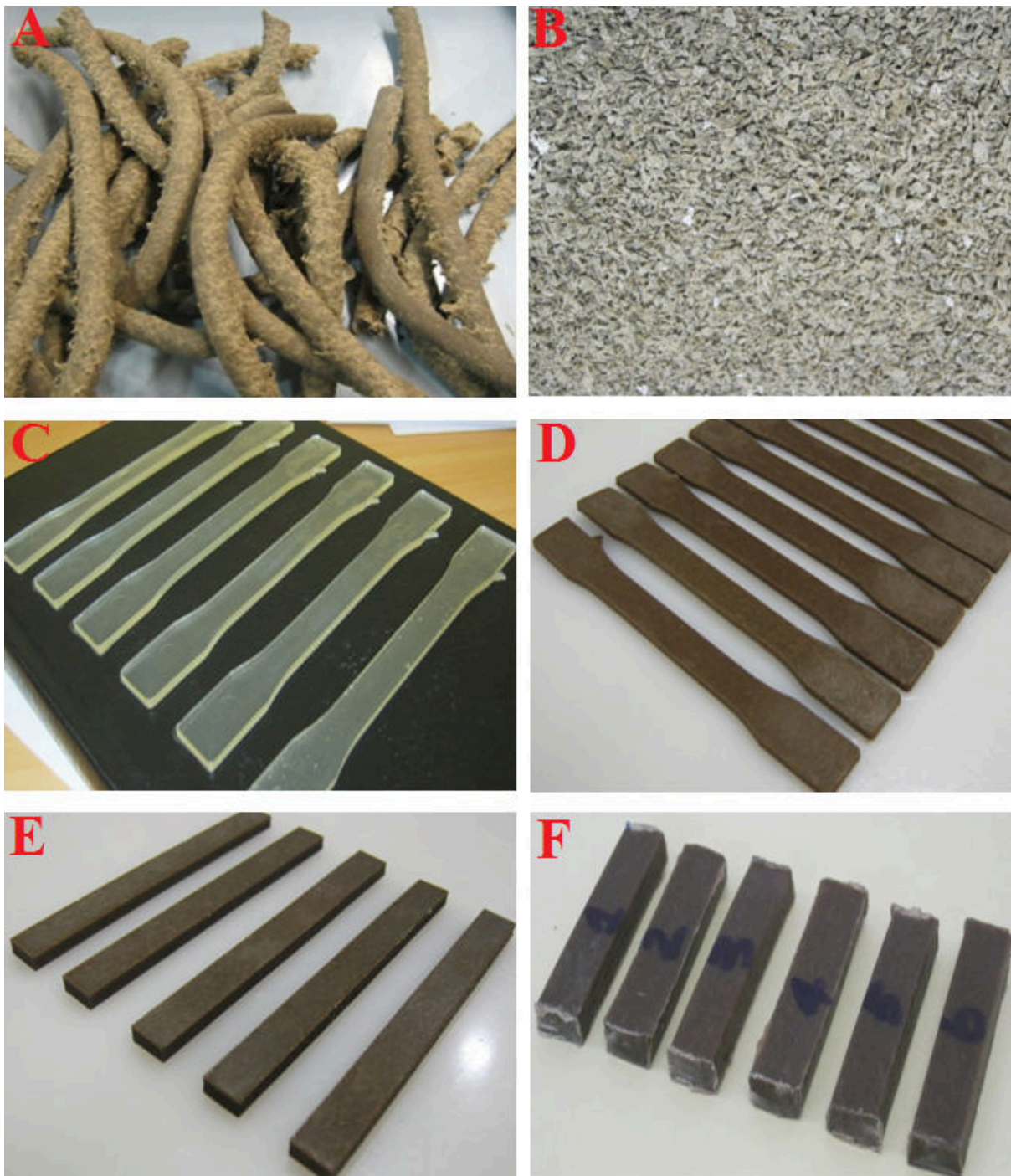
Figure 3. Extruded compounded hybrid composite (A); Granulated extruded compound of hybrid natural fibre and matrix (B); Fabricated tensile test specimens of pristine PLA (C); Fabricated tensile test specimens of Hybrid fibre reinforced with PLA (D); 9 Composite impact test specimens (E) and hybrid composite DMA test specimens (F).
