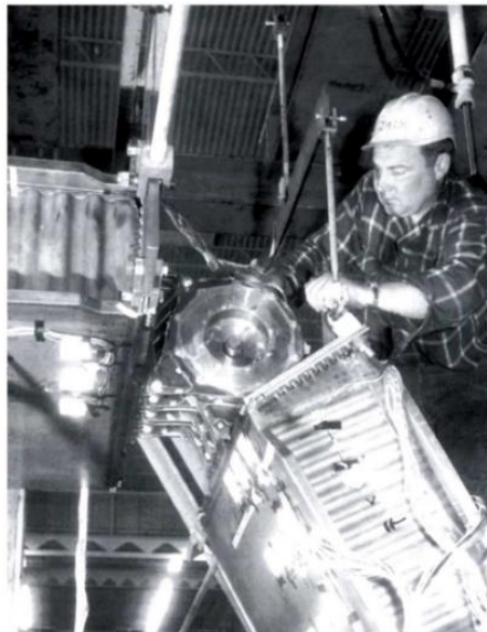
Figure 9. XB-70 power hinge inside the wingbox, with operator for size comparison.
