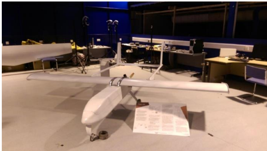
Figure 6. Photograph of model Aegis UAV with U-tail configuration at Cranfield University. The A1 sheet of paper gives an indication of model size.
