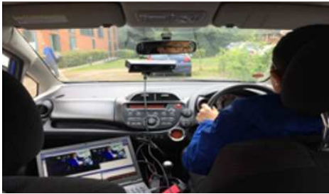
Fig. 2. Experiment setup. The Kinect is mounted on the middle of the front window and data are collected using a laptop.
