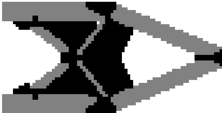
Figure 7 Aluminum occupies 25% of the design domain
