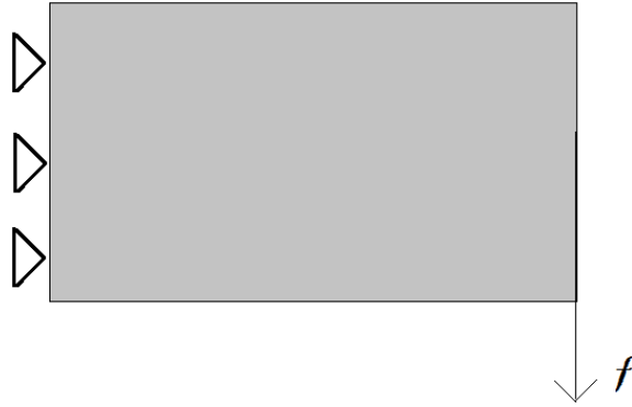
Figure 1 The model of a cantilever beam used as the design domain
