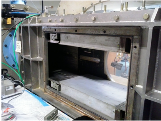
Figure 1: Transonic wind tunnel with side door removed; flow direction right to left.
