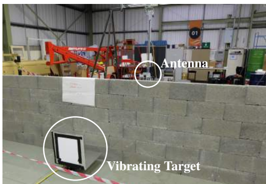
Figure 6: Experimental set-up used for through-wall measurements.
