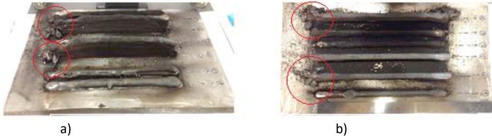
Fig. 5. Wall failures during multiple deposition trials, a) Wall failure due to high heat input (WFS=10 m/min, TS= 1.2 to 1.5 m/min); b) Wall failure due to high end current duration ( \geq 0,2s )
