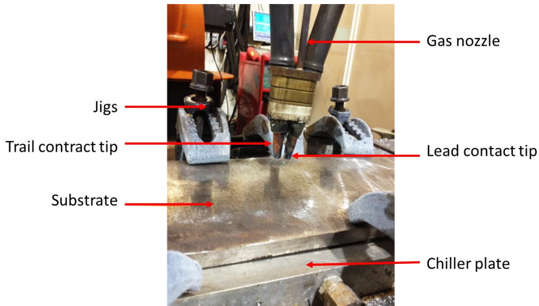
Fig. 3. Tandem torch working configuration
