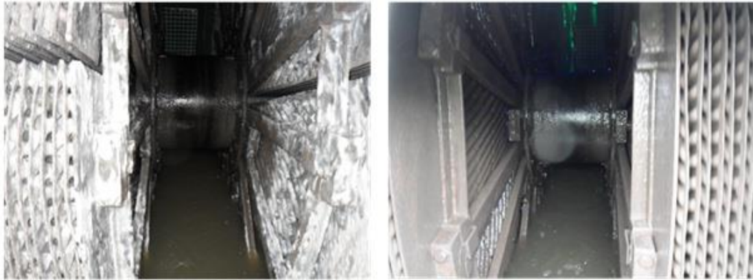
Figure 5. The biofilm at tip speeds of 0.16 (left) to 0.2 m/s (right). Filamentous Beggiatoa bacteria can be seen on the slower RBC, whereas on the quicker RBC the biofilm is thinner and brown.
