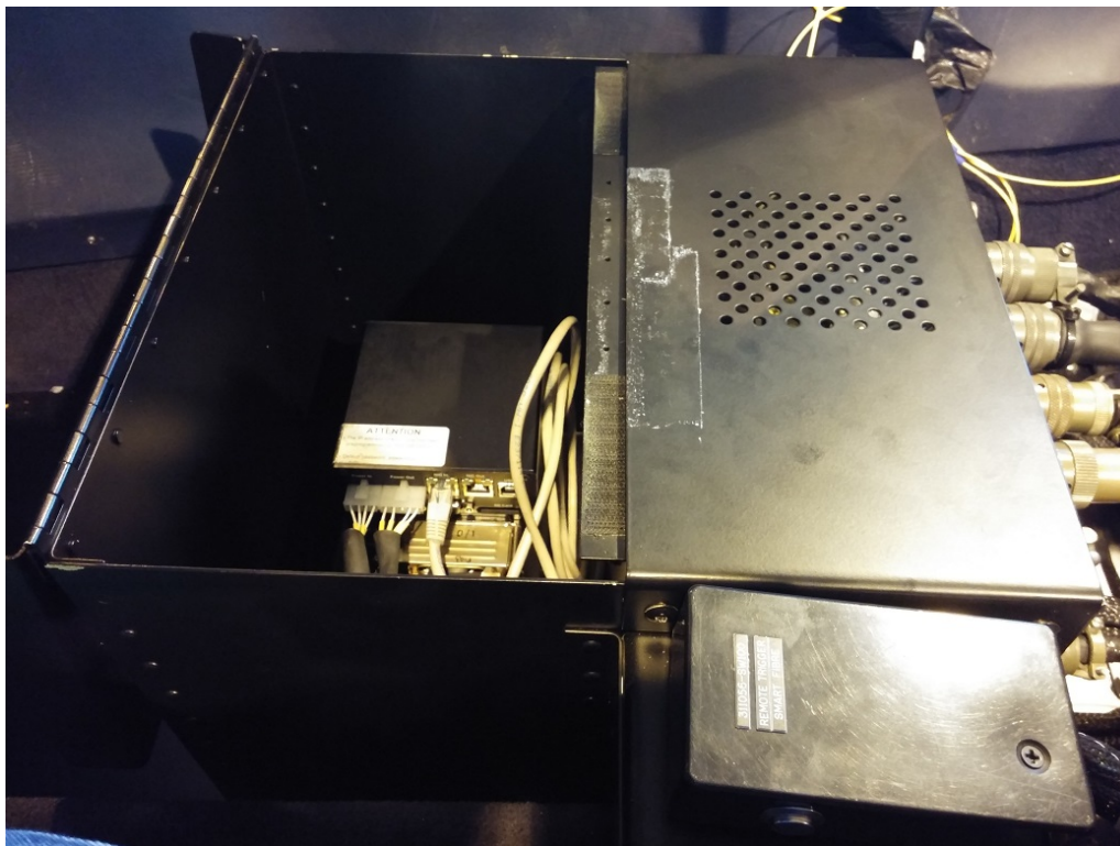
Figure 6.2: Mounting box inside Scottish Aviation Bulldog, with internal dimensions of 300X167X270mm.
