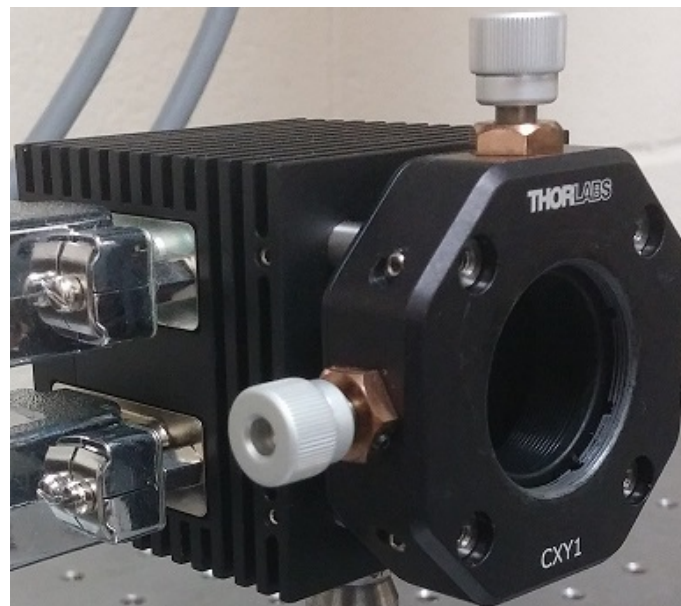
Figure 5.2: Picture of 3311.3nm ICL in Laboratory. The laser is packaged within a large heatsink and collimation optics.
