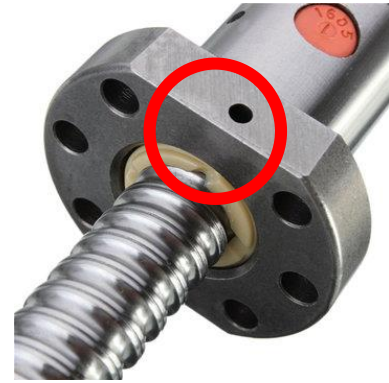
Fig. 5: Bolt holding seal in ballnut
