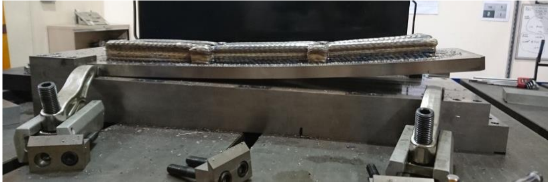
Figure 7 Structural distortion of a WAAM part
