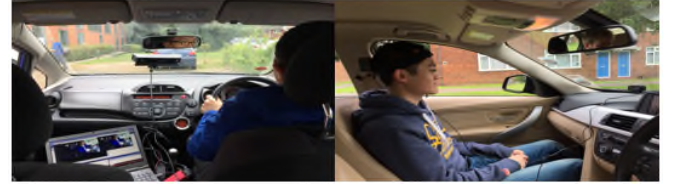
Fig. 3. The left image illustrates the Kinect setup inside the vehicle and right image shows a participant seated in the passenger seat wearing the head tracker.
