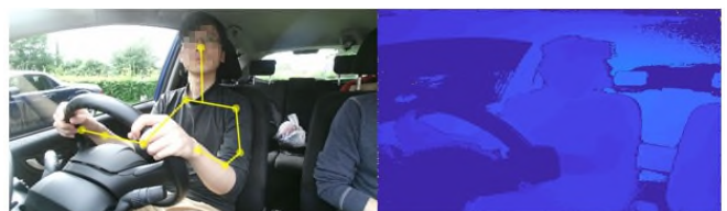
Fig. 2. The left image shows the head and body joints for the seated driver detected using the Kinect sensor. The right image shows the depth image given by Kinect.
