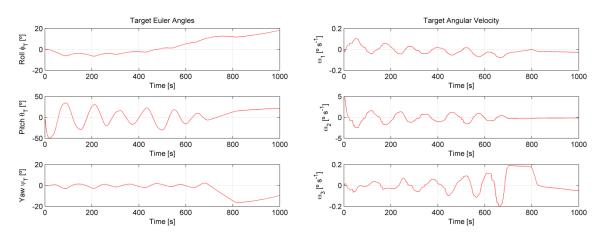
Figure 14: Target attitude and attitude rates - low OBSW frequency case
