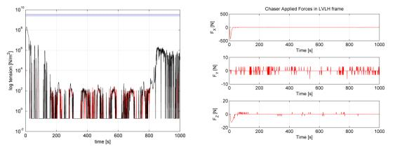
Figure 6: (a) Tether tension, nominal case (b) ADR Chaser forces in LVLH frame, nominal case
