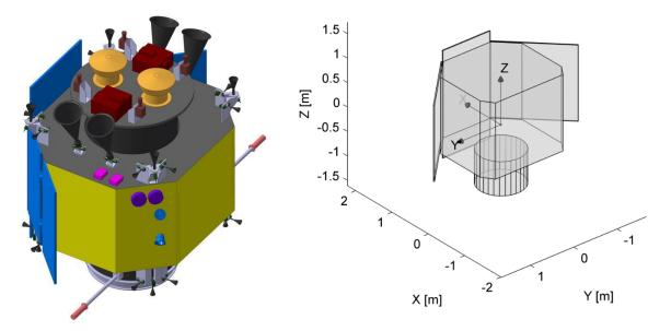
Figure 2: ADR chaser layout and body frame definition [9]
