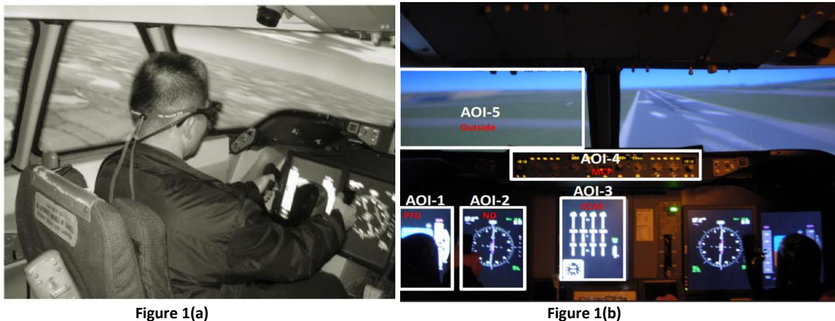
Figure 1(a): Research apparatus including eye tracker and Boeing 747 flight simulator; Figure 1(b): The definition of AOIs: AOI-1(Primary Flight Display); AOI-2 (Navigation Display); AOI-3 (Engine Indication and Crew Alerting System); AOI-4 (Mode Control Panel), and AOI-5 (Outside of Cockpit).
