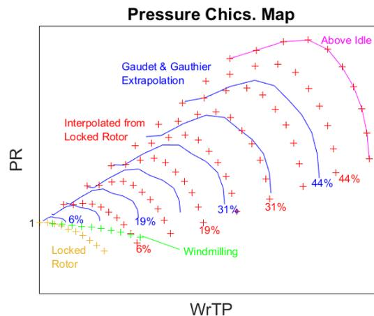
**Figure 7 Comparison of interpolation and extrapolation methods for M250 sub-idle map.**
