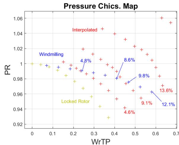
**Figure 9 Interpolated low speed characteristics using windmilling line.**
