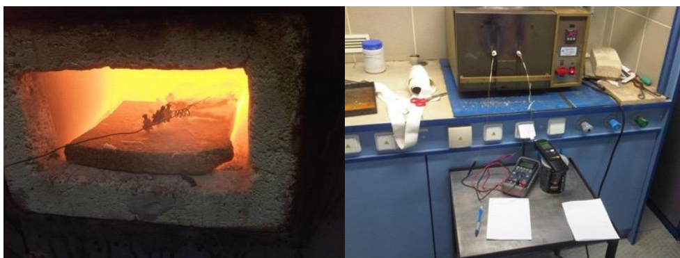
Figure_Apx D-5: Conductivity measurements of the refractory mastic used for the construction of the furnaces
