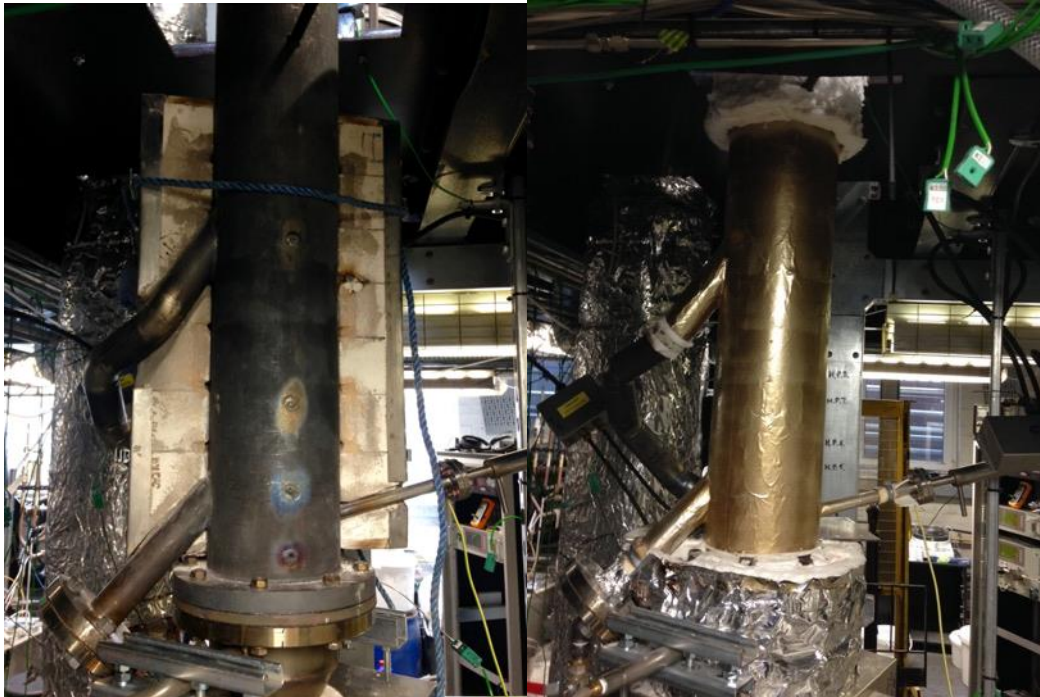
Figure_Apx D-7: Wrapping the calciner by mica sheet (COGEBI Flexible Cogemicanite 132) to protect it from potential electrical discharge from the electrical furnace
