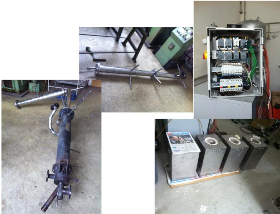
Figure_Apx C-3: Reconstructed calciner and fabricated new parts with new control unit and furnaces ready to be transported to Cranfield University
