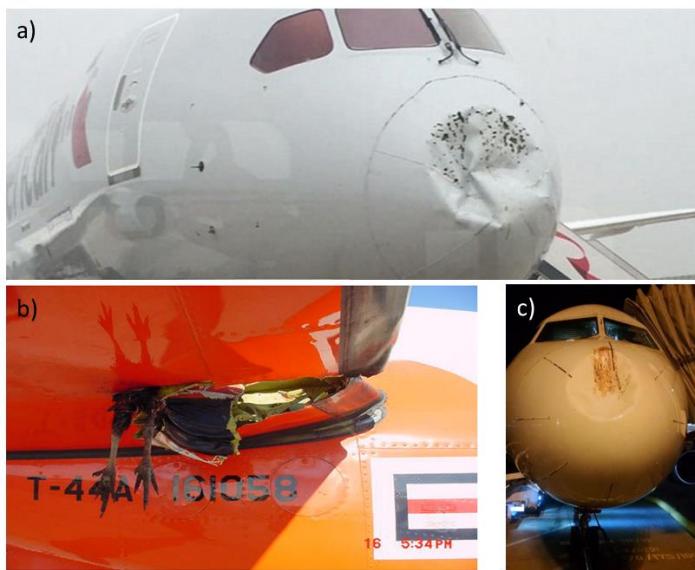
Figure 1.1.1 Plane's fuselage and wings are made largely from carbon-fibre composite (Taken from Ref. 5 ), b) and c) damage due to bird strike (Taken from Ref. 6 )
