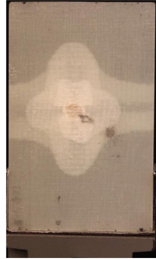
Figure 4.2.18 Impacted specimens with 0% AB before and after UV irradiation
