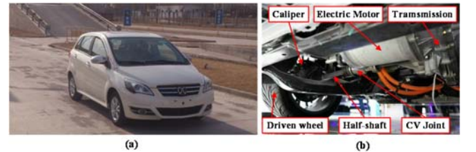
Fig. 3. Pictures of the test vehicle and the electrified powertrain system.
