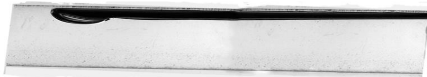
(a) 160cp_0.099m ID pipe_1degree, (LTT)
