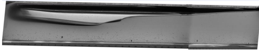
(c) 160cp_0.099m ID pipe_2.5degree_Vso = 0.31m/s
