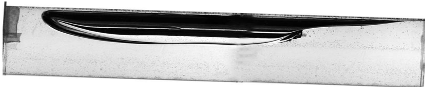
(b) 160cp_0.099m ID pipe_2.5degree, (STT)
