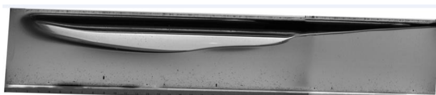
(a) 160cp_0.099m ID pipe_2.5degree_Vso = 0.11m/s
