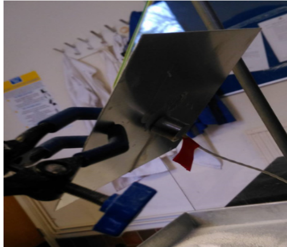
Figure 3: AE Sensor On The Back Of Experimental Target Plate
