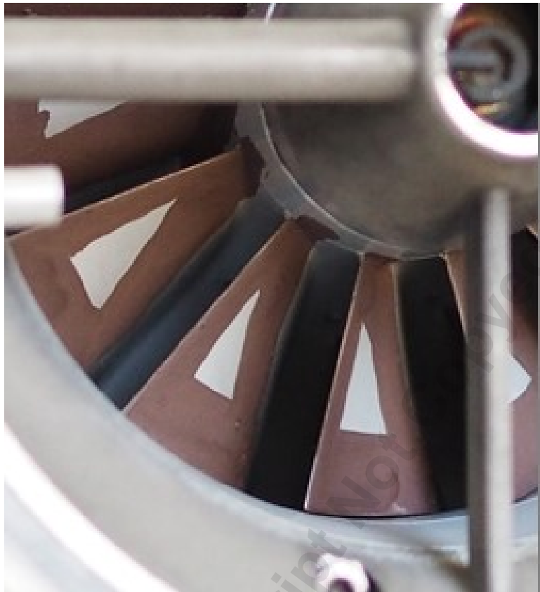
Fig. 2 Simulated fouling pattern in test rig compressor
