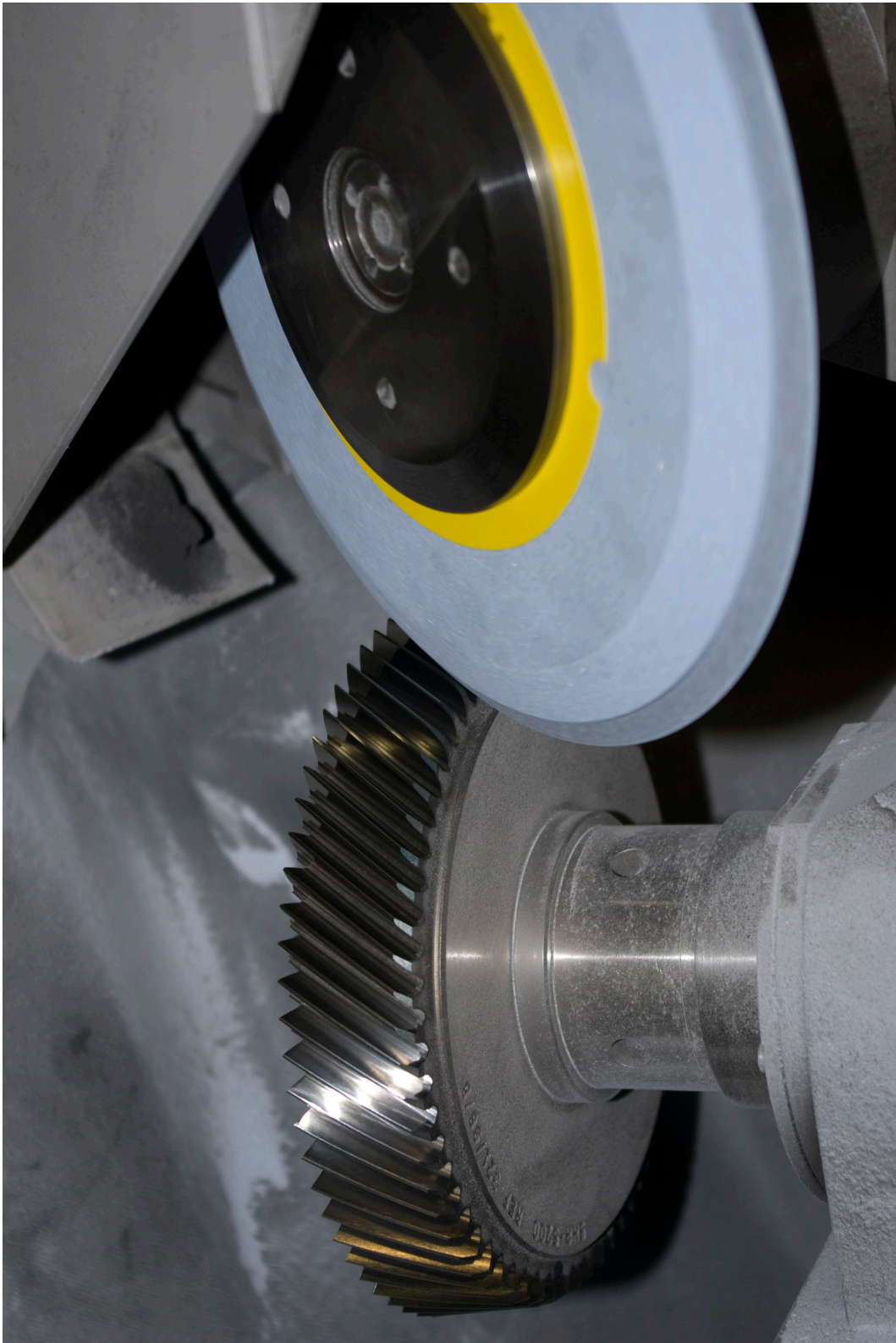
Figure 1.6: Generation of a helical gear shaper cutter with a grinding wheel
