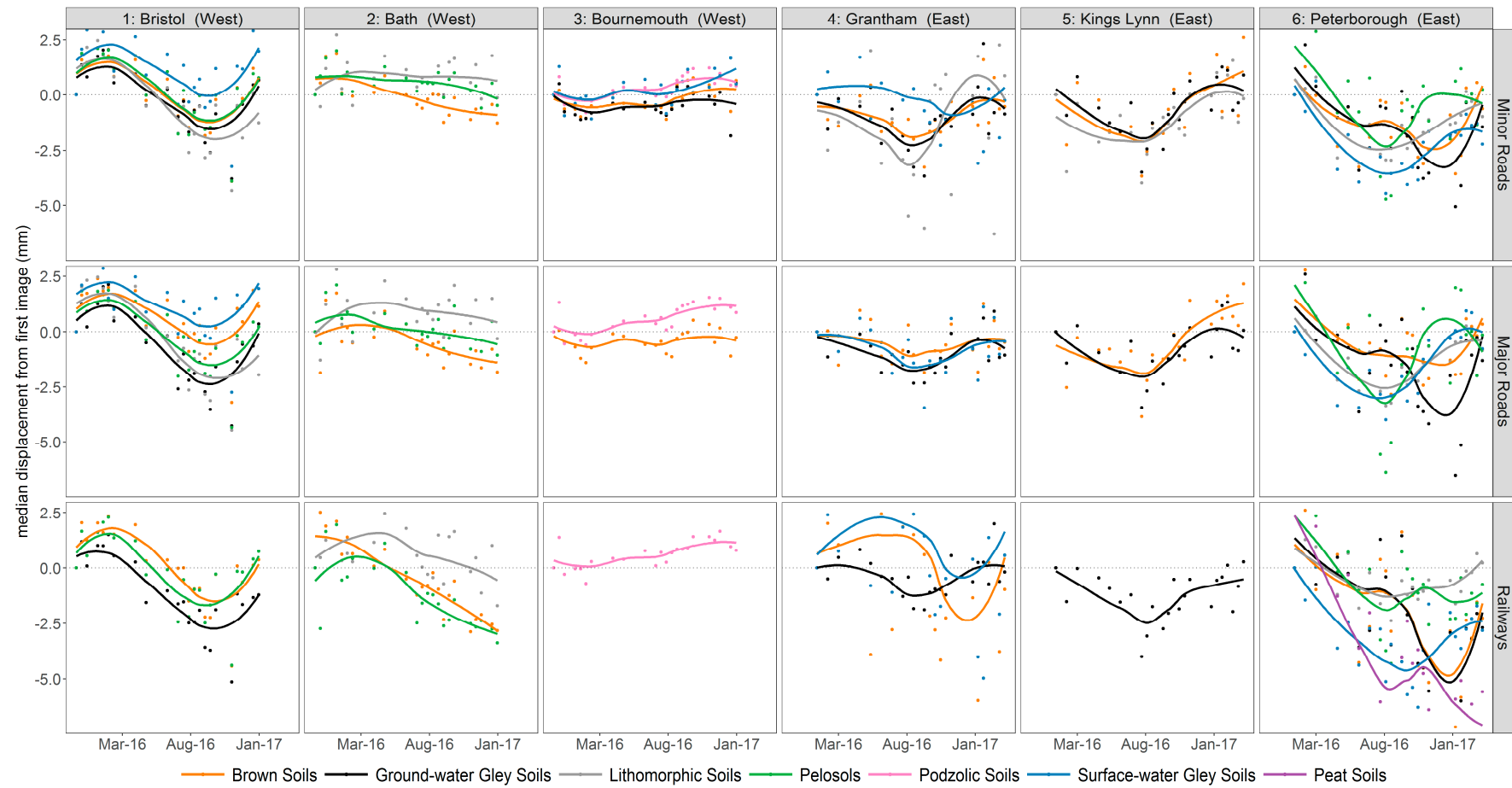
Figure 4. Trends in vertical movement (mm) by major soil group and infrastructure type. Points show median value for all PSI points on an infrastructure type and major soil group. Solid line show a loess-smoothed trend through the plotted medians. Dashed lines identify 1st January. To ensure validity, classes with less than 100 PSI points have been removed from this plot (Table 5).
