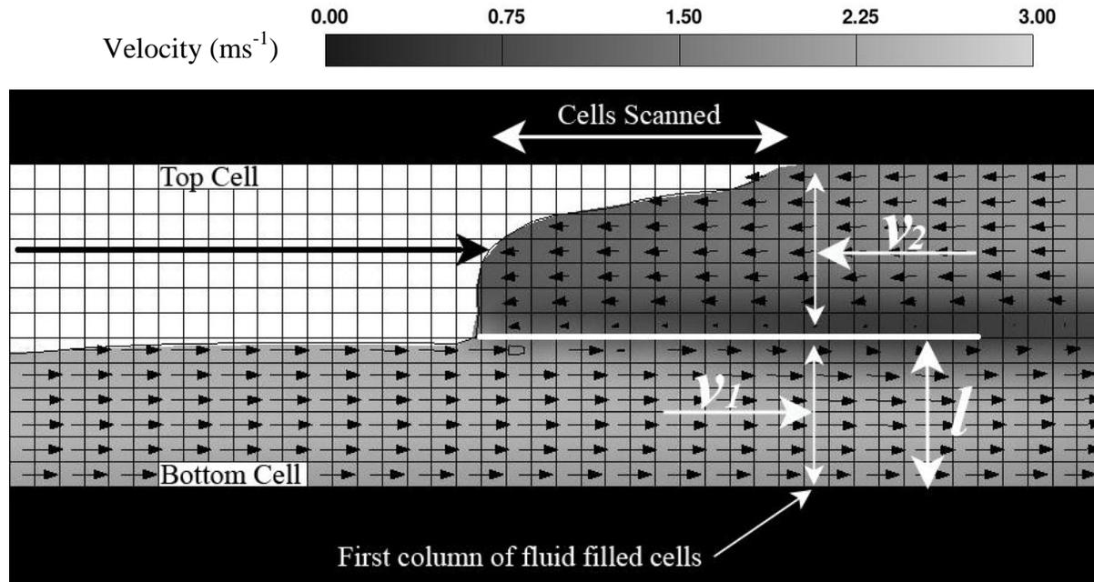
Figure 3. 2D Return wave showing Fr calculation method
