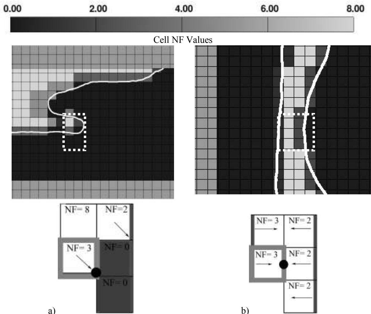
Figure 2. Example of entrainment logic. (Arrows represent velocity vector) a) Returning wave as seen in Figure 8. b) Colliding fronts as seen in Figure 6b.
