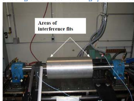
Figure 3—53 Two-disk rotor installed on the ball bearings at the Turbomachinery Laboratory [41]
