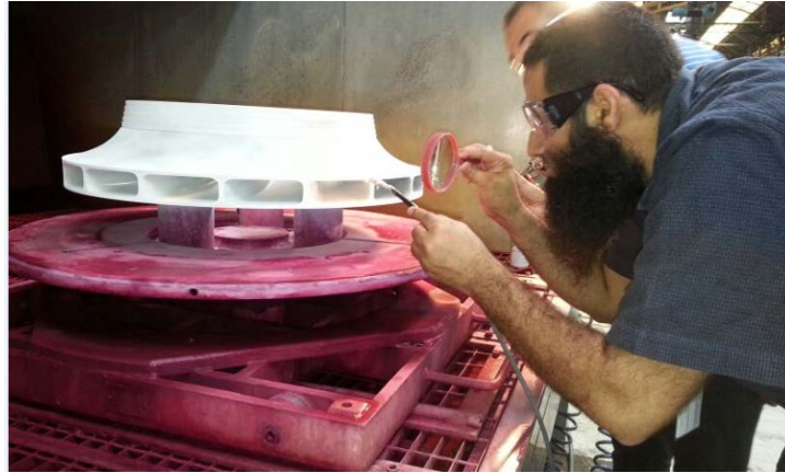
Figure 3—45 Impeller Penetrate test, GE 2014
