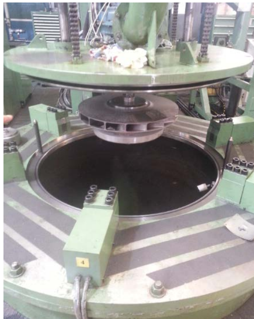
Figure 3—46 Impeller test bunker, GE 2014
