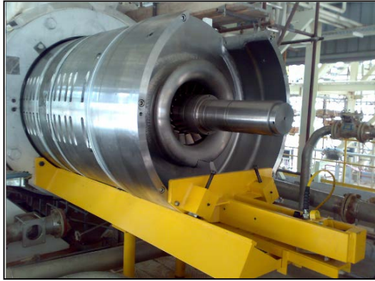
Figure 1—8 Vertical split type (PDO, Harweel plant 2012)
