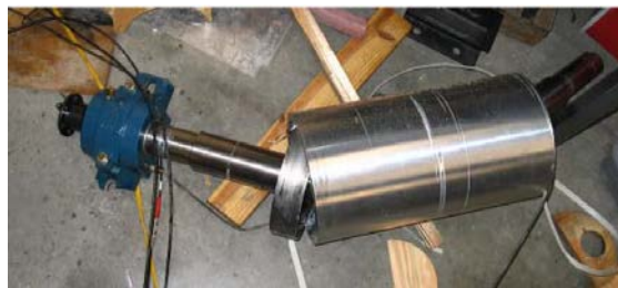
Figure 3—54 the two-disk rotor with an aluminum sleeve shrink fitted destroyed [41]
