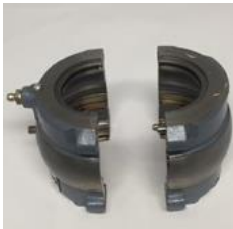
Figure 4.6: Specimen housing (01 BCP 35MM GR ATL)
