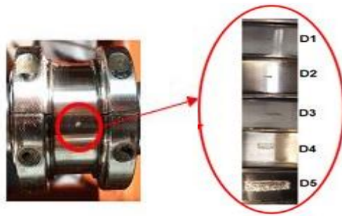
Figure 4.17: Inner race defect severities
