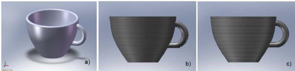
Figure 2-1 CAD image of a teacup building using AM with different layer thicknesses (Gibson et al., 2010)
