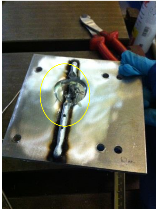
Figure C- 5 Wrong setting of operating program resulted in the broken of workpiece and machining tool
