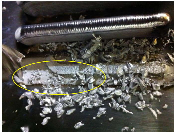
Figure C- 2 Too small WFS (first layer) resulted in low current and small dilution, layer separated from substrate after milling was done
