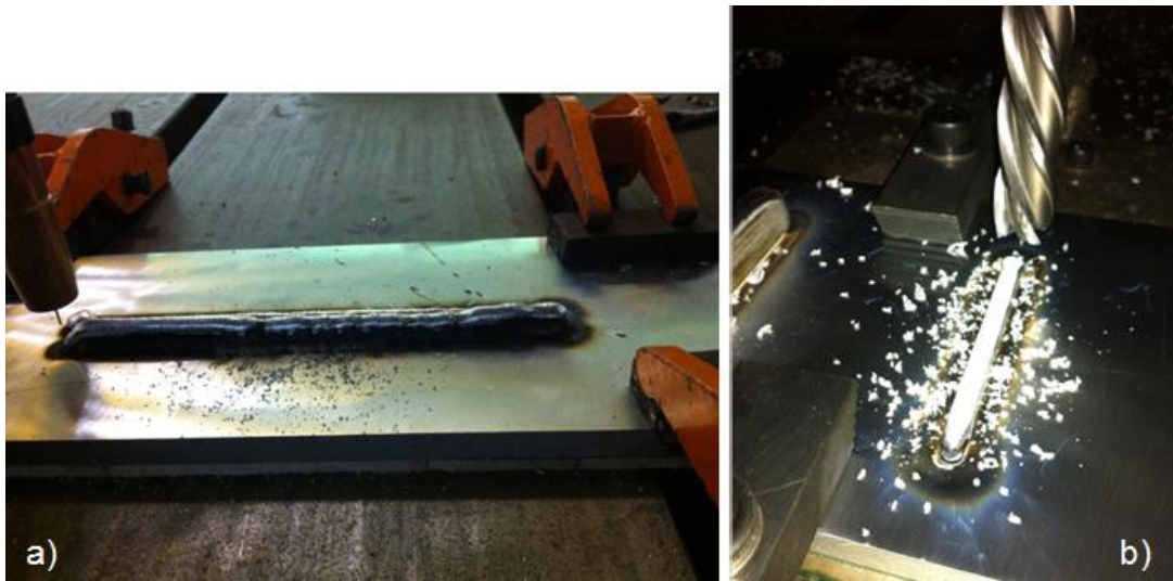
Figure 4-7 Process principle of integrated deposition and machining, a) WAAM process, b) Face milling process
