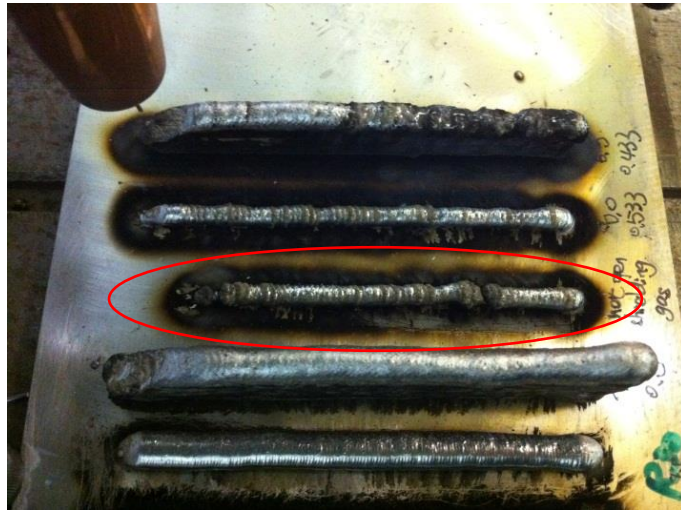
Figure C- 1 Walls got poor quality when there was no shielding gas during the deposition process
