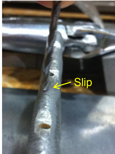
Figure 5-3 Drill slips on the top of weld bead
