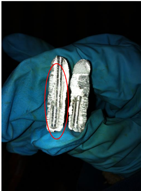
Figure C- 4 Holes present nearly folding line because of drill slipping the top of weld bead
