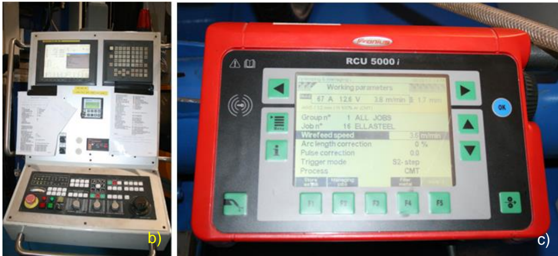
Figure 4-1 WAAM systems: a) HiVE machine b) Control console c) RCU 5000i control pendant
