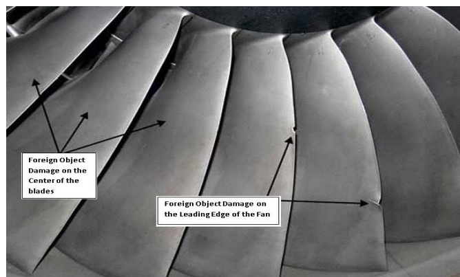
Figure 3-6 FOD of a fan blade (Yupu 2008)
