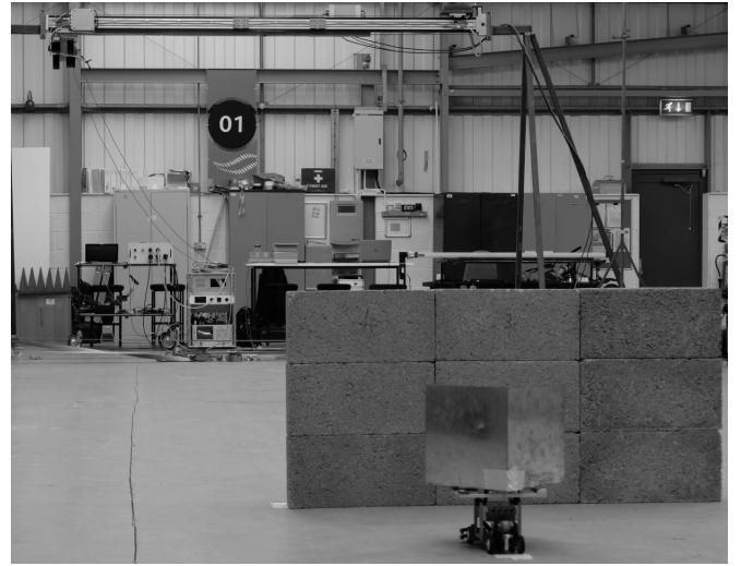
Fig. 5 Experimental measurement scene set up. The 876 \times 645 [mm] breeze block wall is situated 10 [m] down range from the radar antenna horns, on the SAR scanner. The vibration rover with situated trihedral is located 1 [m] behind the wall.
