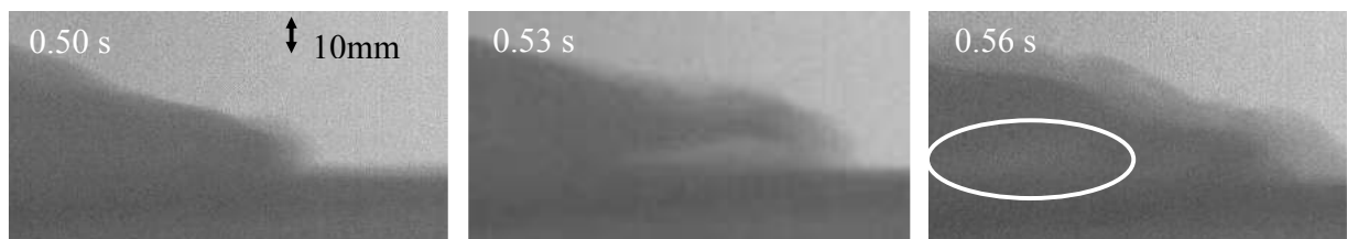
Figure 8. Instability in advancing flow front leading to entrainment of an air bubble; Trial 2
