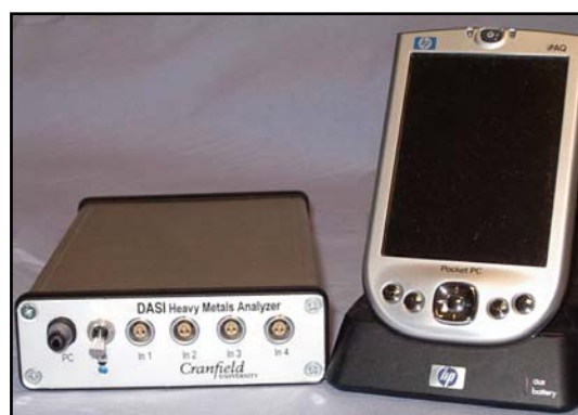
Figure 4.2: In-house custom-built multi-channel potentiostat and Pocket PC PDA
