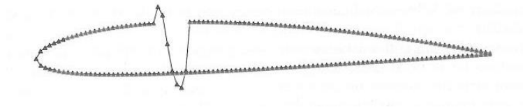
Figure 2-1 Changes in an airfoil described by a series of points (Keane and Nair, 2005)
