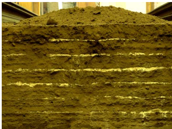
Figure 23 Photograph of the 'bow wave' (top) caused by the tyre pushing the soil in front of it along
