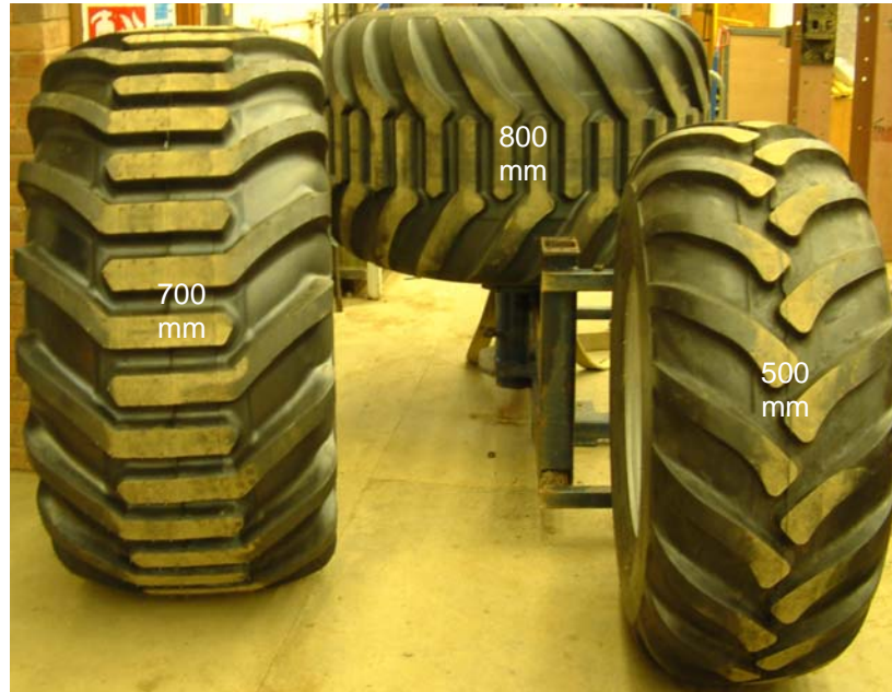
Figure 4 The three tyres used during the study showing section width and tread pattern
