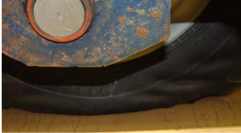
Figure 12 Tyre wall flexing of the 800 mm tyre inflated to 0.9 bar caused by the tyre operating below the manufacturers' recommended inflation pressure for the applied load
