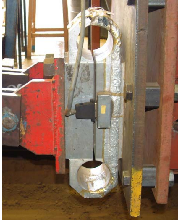
Figure 6 The Extended Octagonal Ring Transducer used in this study to measure rolling resistance attached to the Soil Bin Processor
