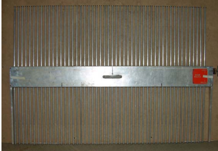
Figure 7 Profile meter used to determine the soil deformation at the surface after each test during the study
