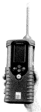
Figure 2.8.3.5 Photograph of Cyranose 320 portable sensor array monitor (Courtesy of Cyrano Sciences, USA).
